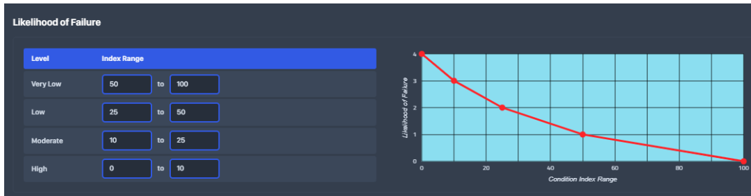
Figure 6: Likelihood of Failure Setting
